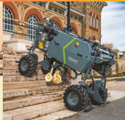
EXXACT Robotics' TRAXX compact autonomous single-row high-clearance tractor
